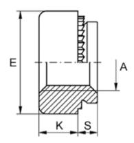
Female thread A = M4Height K = 2.0Max recess height = 1.0 Min distance to edge = 4.0Outer diameter E = 8.0
